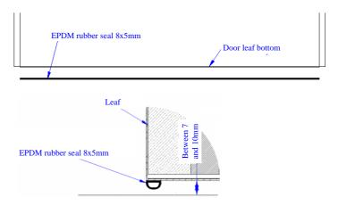
COMMENT: It's very important to leave between 7 and 10 mm between the bottom of the door leaf and the floor. If not, the door will not close properly.
