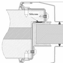
2. Un-install the porthole and fit silicone between the glass and the rock wool (see the drawing). Then install the porthole.
